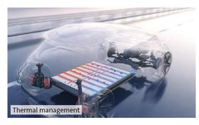
number of pumps, valves, and flaps throughout the vehicle, thus maintaining an optimal operating temperature for all mechanical and electronic components. This increases the efficiency of the drive system and reduces energy and fuel consumption.
