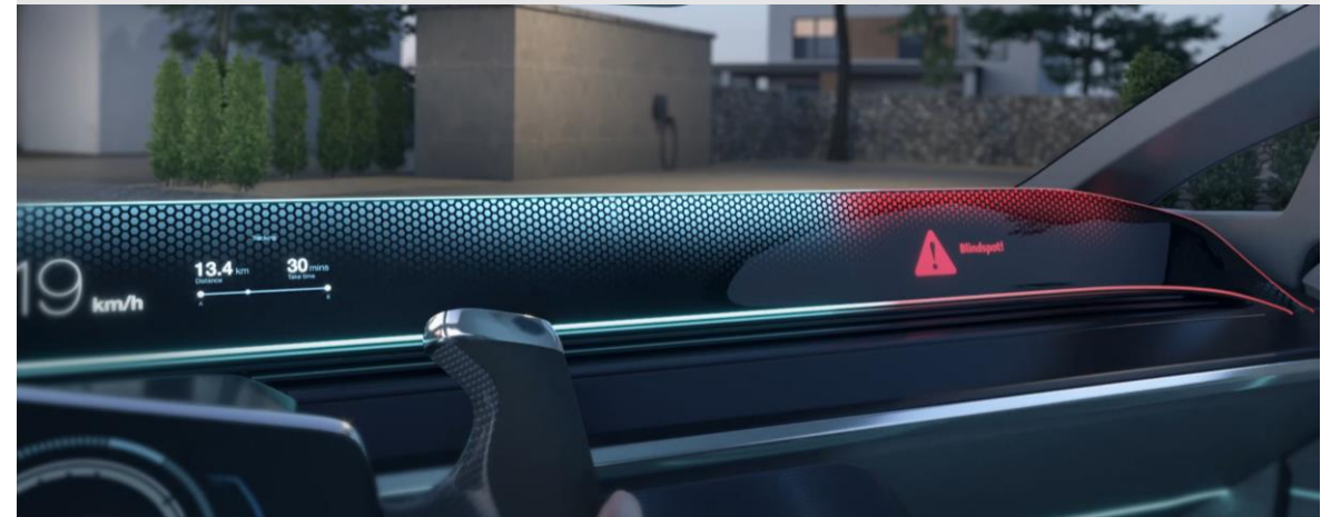
Dashboard Ambient Light Control for Safety Warnings
